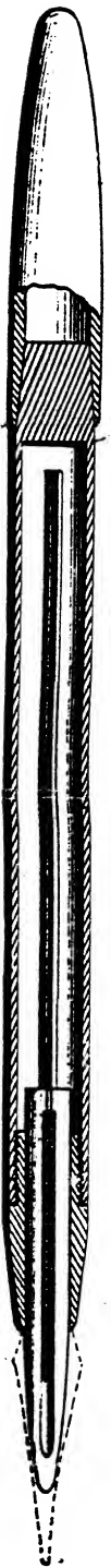
(Fac. Simile of Cooley Patent Pen—Sectional View. Showing taper cap and joint.) Issued years before the Inventor (?) Waterman's.
